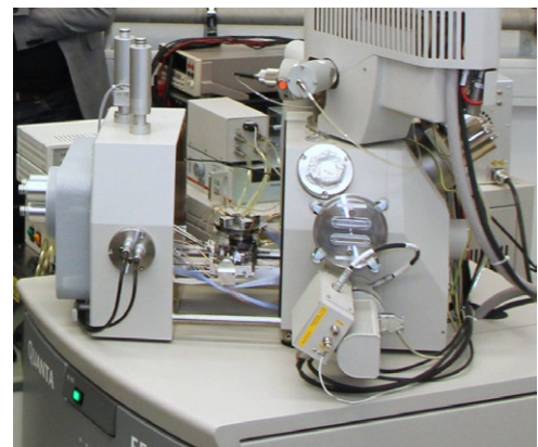
Figure 2: Photograph of the FEI Quanta 650 ESEM that was used for the experiments.
