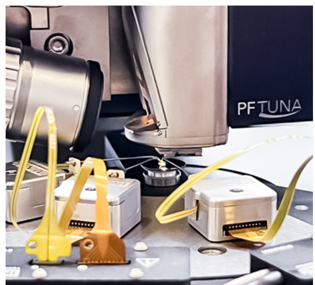
Figure 1. Imina Technologies' miBot™ nanoprobers positioned onto a small sample (mounted on a SEM-compatible stub) on the Bruker Dimension Icon® AFM equipped with the PeakForce TUNA™ application module.
