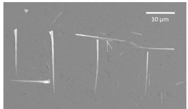
Figure 1. Manipulation of single ZnO nanowires into an arrangement that spells the abbreviated university name (UTT). (Source: [1])
